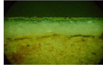
Figure 18a- Part of a longitudinal cut in a shivered tile showing a glaze delamination over a recess that does not reach the edges (marked by a grey line); 18b- detail under the optical microscope
